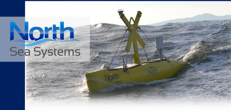
DataFish® is North Sea System's metocean survey buoy for unforgiving marine environments. By providing real time data and undertaking long duration, multi-application surveys, the system reduces the risk and cost of metocean data collection. DataFish® is the only system able to provide real time data from tidal energy sites.
